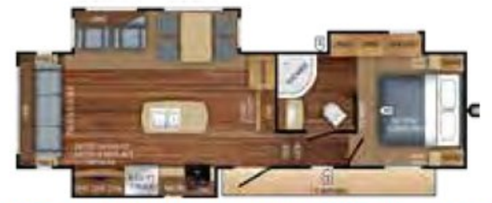
EAGLE HT FIFTH WHEEL | 28.5RSTS OPTIONS: A, E Ext. Lgth: 33' 0" Ext. Ht: 143**** Unloaded Wt. (lbs): 8,600 Sleeps: 4-6
