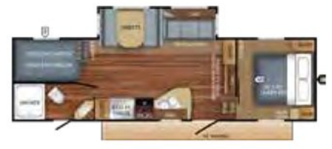
EAGLE HT FIFTH WHEEL | 26.5BHS OPTIONS: B, D Ext. Lgth: 31' 7" Ext. Ht: 150" Unloaded Wt. (lbs): 7,510 Sleeps: 7-10
