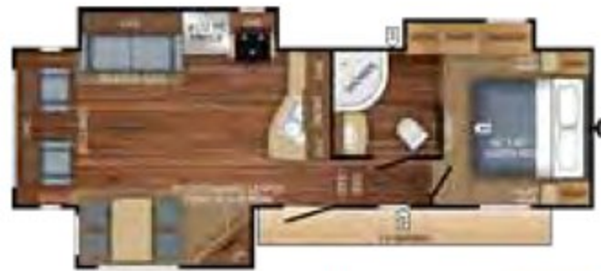
EAGLE HT FIFTH WHEEL | 27.5RLTS OPTION C Ext. Lgth: 31' 2" Ext. Ht: 144" Unloaded Wt. (lbs): 8,045 Sleeps: 4-6
