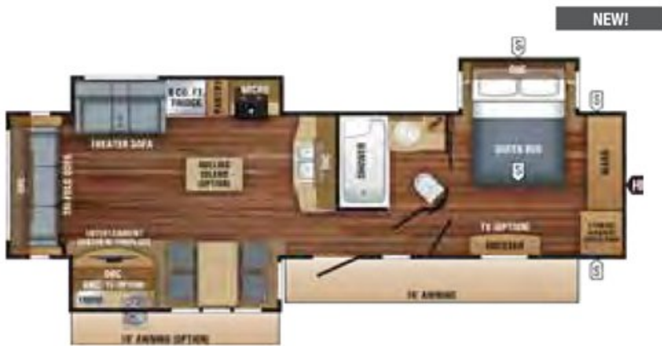
EAGLE TRAVEL TRAILER | 322RLOK OPTIONS: E, G Ext. Lgth: 38' 5" Ext. Ht: 146" Unloaded Wt. (lbs): 9,505 Sleeps: 4-6
