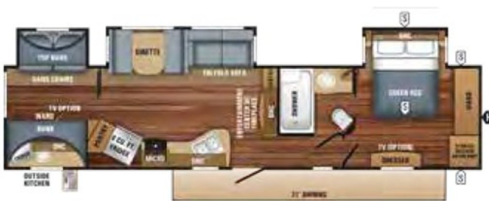
EAGLE TRAVEL TRAILER | 333BHOK OPTIONS: B, D, E, G, H Ext. Lgth: 41' 7" Ext. Ht: 142" Unloaded Wt. (lbs): 10,250 Sleeps: 7-10
