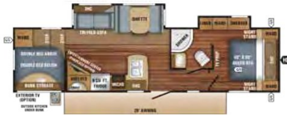
EAGLE HT TRAVEL TRAILER | 295DBOK OPTIONS: B, F, H Ext. Lgth: 37' 10" Ext. Ht: 138" Unloaded Wt. (lbs): 8,425 Sleeps: 7-10
