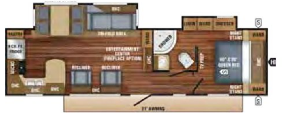
EAGLE HT TRAVEL TRAILER | 306RKDS OPTIONS: A, C Ext. Lgth: 35' 9" Ext. Ht: 138" Unloaded Wt. (lbs): 7,865 Sleeps: 4-7
