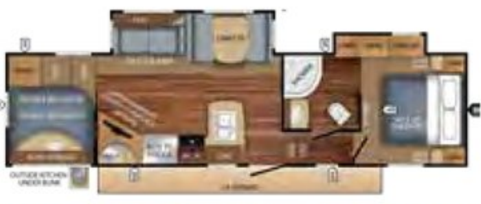
EAGLE HT FIFTH WHEEL | 29.5BHDS OPTIONS: B, D, E Ext. Lgth: 34' 9" Ext. Ht: 149**** Unloaded Wt. (lbs): 8,655 Sleeps: 7-10
