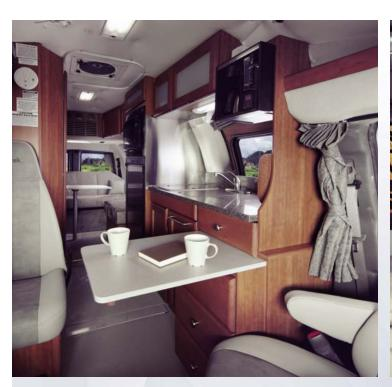
The 210-Popular's expanded galley has a larger window and a longer and deeper engineered granite counter. A convection/microwave oven and 5 cu.ft. refrigerator are located after the galley to create more space for a handy pull-out table, four deep drawers and a huge cupboard below the counter. The twin beds are wider (30") and the king bed is wider as well (6'8").
