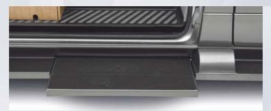
RS and SS models feature a power step at the side entry that extends/retracts with the opening and closing of the sliding entry door. An override switch allows the step to be left extended while parked. Sensors ensure the step retracts when driving.
