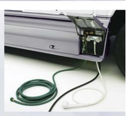
There is a separate compartment for the city water connection with quick disconnect and detachable power cord for trips away from the campsite. An exterior shower is located here as well.
