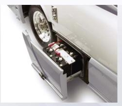
190-Popular, 210-Popular and Sprinter based models feature two auxiliary deep cycle 6V AGM batteries with 220 total amp hours. On 190 and 210 models they're located on a convenient slide-out tray.
