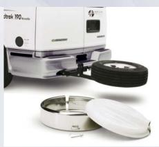
Optional Continental kit looks great and provides more interior storage. It's mounted on the receiver to avoid stress and rust on the door and off centre to the trailer hitch to allow towing, receiver mounted bike racks and access to one door. To access the other door, simply remove the hinge pin to lower the spare tire. To access the tire, just unclasp the tire cover.
