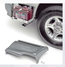
On the 170-Versatile (shown), 190-Simplicity and 210-Simplicity, a large capacity auxiliary 12V AGM battery is totally concealed yet easily accessible on slide-out tray.
