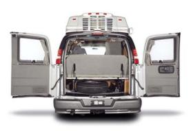
Dual rear doors allow for easy rear loading and swing a full 180° on 170 and 190 models and 270° on RS and SS models.
