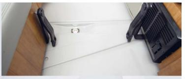
A removable cover in Chevy based Roadtreks reveals a trough with a drain that spans the lowered floor and prevents water from leaving the shower area.
