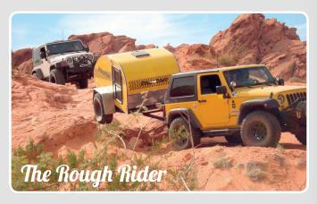
Beef up any Little Guy for the ultimate off road experience. The Rough Rider features electric brakes, a custom made chassis, pintle hook and skidplates. For that extra bit of performance, we outfit it with knobby 15" mud tires and squared off fenders.
