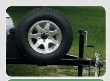
**Spare Tire**Be prepared for a flat: stores on the tongue or under the trailer.
