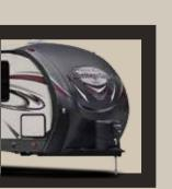
PAINTED GEL COAT FIBERGLASS FRONT CAP WITH LIGHT STRIPS ON LITE SERIES TRAVEL TRAILERS AND FIFTH WHEELS, WON'T FADE, CHALK OR CRACK
