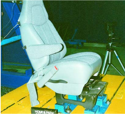
Seating system testing minimizes the possibility of failure of the seats, their attachments and their installation.
