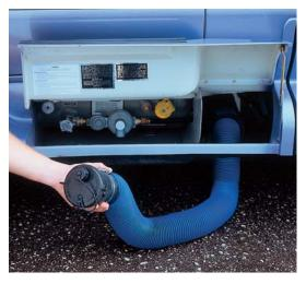
Easily accessible by flipping up the driver's door step, our patented "Dura Drain" sewage hose system provides a permanently attached sewage hose that eliminates messy handling and storage. Also located here are the waste water tank releases, LP gas fill and gauge plus the fresh water tank drain.
