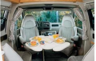
The cab is also living area for eating or entertaining. Our patented cloverleaf table with extendible leaves combines the large surface area of a kitchen table with the compact convenience of a smaller table.
