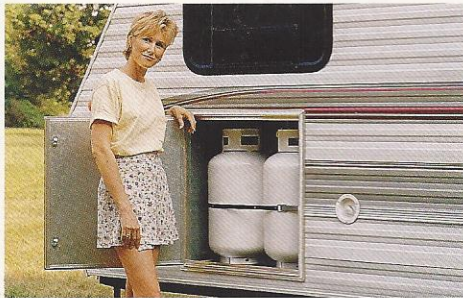
Dual LP-gas bottles, stowed in their own easy-to-get-at compartment on the side of the RV
