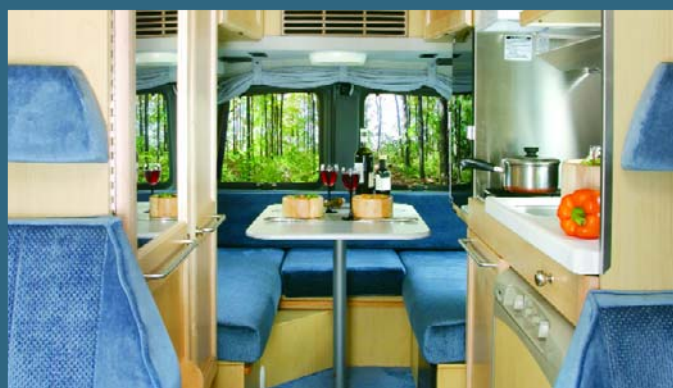
The galley is equipped with 3.0 cu. ft. refrigerator, microwave oven, LP gas stove, exhaust fan, and sink. At the rear, choose a dinette, or L-shaped lounge with cabinet for audio/video equipment and/or storage.
