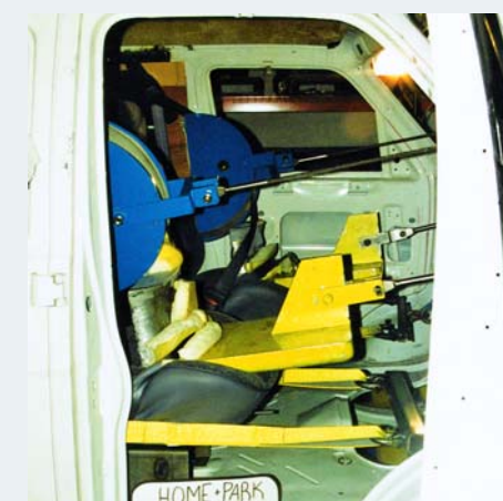
These 2 photos depict simultaneous seat belt pull testing and seating system testing. Seat belt testing confirms proper seat belt location and minimizes the possibility of anchorage failures. Seating system testing verifies the integrity of the seats, their attachments, mounting hardware and installation.
