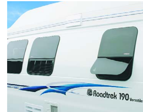
Frameless awning windows are better looking, reduce wind noise, improve aerodynamics, and provide superior air circulation even during foul weather. Their larger size provides a better view from inside. The Integrated Venting System provides inconspicuous ventilation of the refrigerator.
