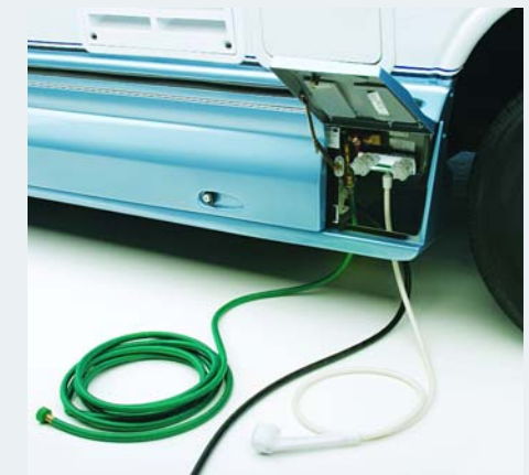
There is a separate compartment for an exterior shower and city water connection with quick disconnect. The 210 features a detachable power cord for trips away from the campsite.
