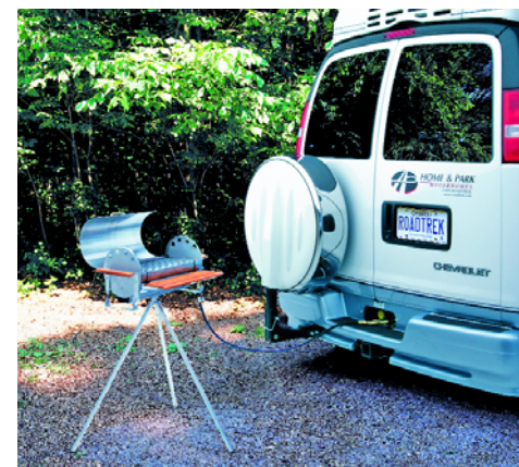
External LP gas barbecue connection with quick disconnect.
