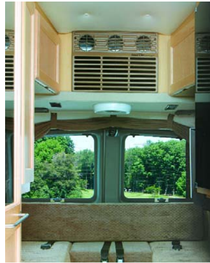
The heat pump (air conditioner & heater) with ducts to the front and rear bed areas is mounted outside for easy service access and external water drainage.
