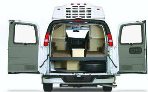
Dual rear doors allow for easy rear loading or egress and swing a full 180 degrees on 170 and 190 models.
