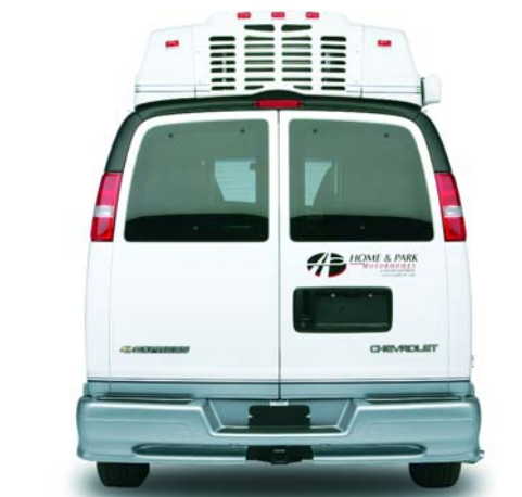
A 'Dometic' heat pump (air conditioner & heater) built into a recess in the roof cools the interior while maintaining Roadtrek's aerodynamic shape and sleek roofline.
