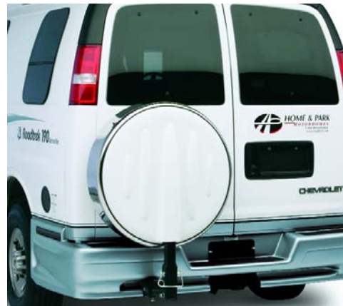
Optional Continental kit looks great and provides more interior storage. It's mounted on the receiver to avoid stress and rust on the door and off centre to the trailer hitch to allow towing and access to one door. To access the other door, simply remove the hinge pin to lower the spare tire. To access the tire, just unclasp the tire cover.
