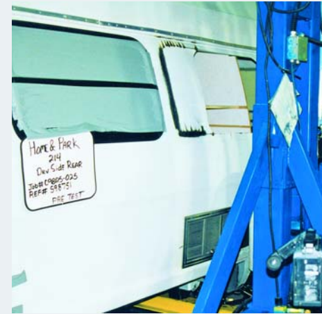
These photos depict side crush resistance testing which is intended to simulate the vehicle impacting a utility pole at a perpendicular angle.
