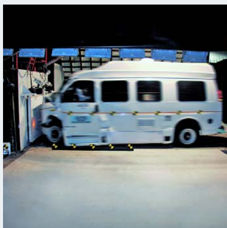
For frontal impact testing, the test vehicle impacted a fixed barrier at 30-mph (48 km/h). Again our test vehicle did not leak any fuel.
