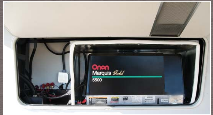
Generator prep with 30 gallon fuel tank standard 5.5 Onan gas generator with second 30 gallon fuel tank (optional)
