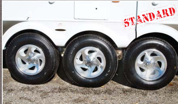
18,000 lb. GVWR and 16" aluminum rims with radial tires 6,000 lb. Triple axle design with shock absorbers
