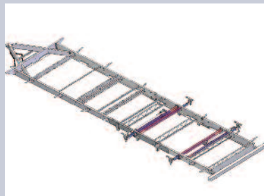
Norco NXG chassis featuring E-Coat technology
