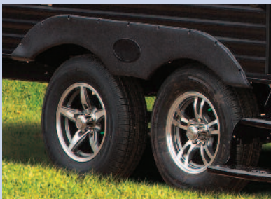
Tandem axles enhance stability
