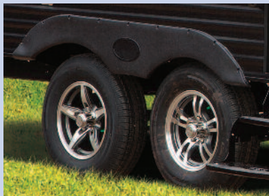
Tandem axles enhance stability
