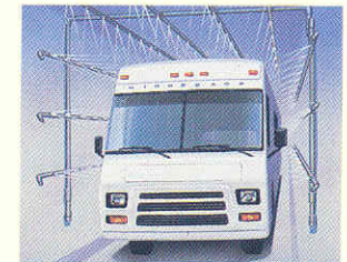
A water test is conducted at the end of the assembly line to make sure each unit is watertight. We use 160 spray heads to simulate an intense rainfall.
