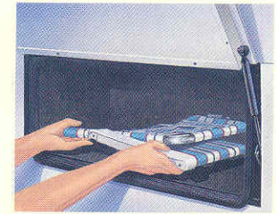
Hinged valance panels held open by gas struts allow easy access to most exterior storage compartments. The single latch can be opened with one hand.
