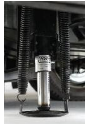
The HWH fully automatic hydraulic four-point leveling system is standard on the F-Series.
