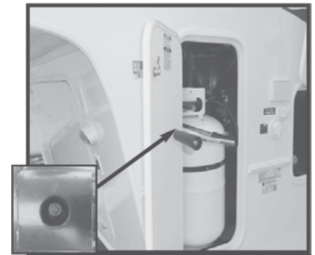
5th Wheel Landing Gear manual operation insert Crank Handle into Actuator Opening located inside the LP Compartment
