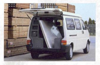
For maximum cargo capacity, both bench seats can be easily removed without tools. Large door openings and an extended wheelbase allow for all sorts of load capabilities, including 4' x 8' sheets. At only 80 inches tall, the EuroVan Camper fits into most conventional garages and parking facilities.
