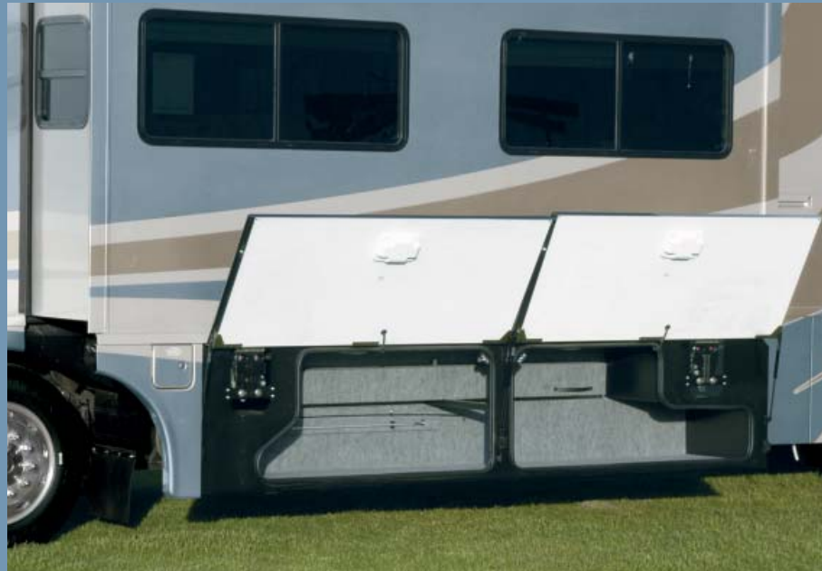
WEB STOREMORE The StoreMore slideout system allows exterior storage compartments to move with the slideout for easy access to your gear.
