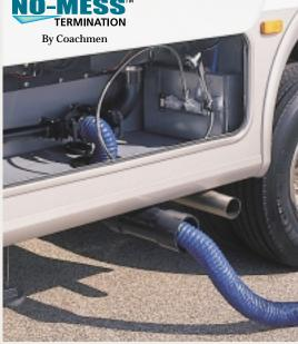
The Coachmen exclusive <u>No-Mess</u><sup>™</sup> termination system is an easy to swivel boom arm that provides a convenient storage location for the termination hose. Your storage bay stays cleaner and the hose can remain connected after use. ALUMICAGE
