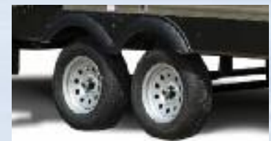
Grey steel wheel rims with Super Lube axles and ABS molded fender skirts
