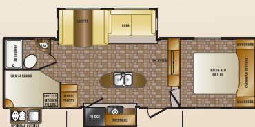
SF270BH — SUPER LITE FIFTH WHEEL EXTERIOR LENGTH: 28' 6" / EXTERIOR HEIGHT W/ AC: 12' 7" / HITCH WEIGHT: 1030 / AXLE WEIGHT: 5554 / UNLOADED WEIGHT: 6584 / CARRYING CAPACITY: 3046 / TIRES: 225/75R15D
