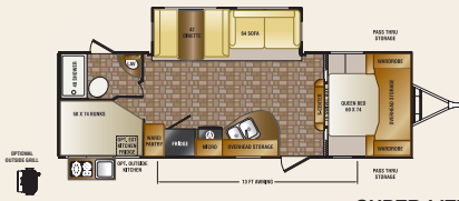
ST270BH — SUPER LITE TRAVEL TRAILER EXTERIOR LENGTH: 30' 1" / EXTERIOR HEIGHT W/ AC: 11' 2" / HITCH WEIGHT: 556 / AXLE WEIGHT: 4798 / UNLOADED WEIGHT: 5354 / CARRYING CAPACITY: 1965 / TIRES: 205/75R15C
