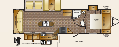
ST32RL — RESERVE TRAVEL TRAILER EXTERIOR LENGTH: 35' 11" / EXTERIOR HEIGHT W/ AC: 11' 4" / HITCH WEIGHT: 998 / AXLE WEIGHT: 6575 / UNLOADED WEIGHT: 7573 / CARRYING CAPACITY: 2025 / TIRES: 225/75R15D
