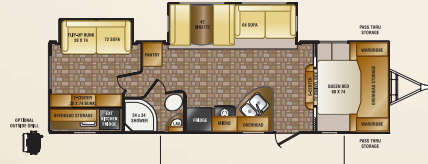
ST300BH — SUPER LITE TRAVEL TRAILER EXTERIOR LENGTH: 33' 2" / EXTERIOR HEIGHT W/ AC: 11' 2" / HITCH WEIGHT: 538 / AXLE WEIGHT: 5538 / UNLOADED WEIGHT: 6076 / CARRYING CAPACITY: 1225 / TIRES: 205/75R15C
