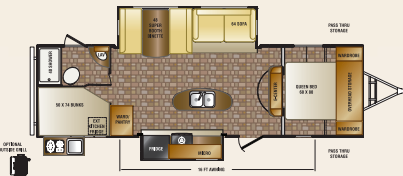
ST28BH — RESERVE TRAVEL TRAILER EXTERIOR LENGTH: 32' 2" / EXTERIOR HEIGHT W/ AC: 11' 2" / HITCH WEIGHT: TBD / AXLE WEIGHT: TBD / UNLOADED WEIGHT: TBD / CARRYING CAPACITY: TBD / TIRES: 225/75R15D
