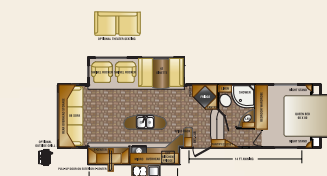
SF32RL — RESERVE FIFTH WHEEL EXTERIOR LENGTH: 33' 11" / EXTERIOR HEIGHT W/ AC: 12' 7" / HITCH WEIGHT: 1898 / AXLE WEIGHT: 6674 / UNLOADED WEIGHT: 8572 / CARRYING CAPACITY: 3486 / TIRES: 225/75R15D
