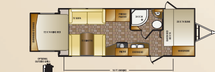
ST230RS — SUPER LITE TRAVEL TRAILER EXTERIOR LENGTH: 26' 0" / EXTERIOR HEIGHT W/ AC: TBD / HITCH WEIGHT: 538 / AXLE WEIGHT: TBD / UNLOADED WEIGHT: TBD / CARRYING CAPACITY: TBD / TIRES: 205/75R14C
