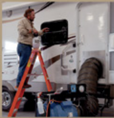
Seal Tech Air Pressure Test
