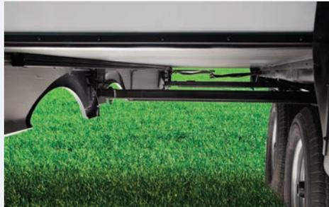
Reliable rack and pinion flush-floor slide system
