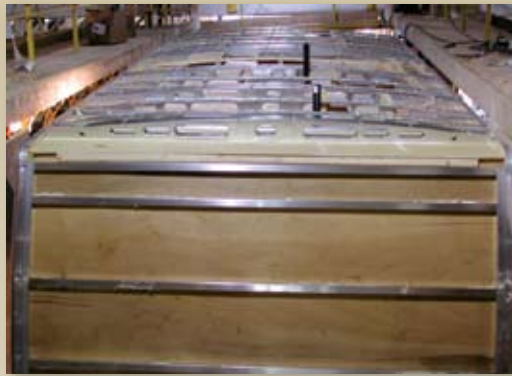
Outback utilizes light weight, long lasting, aluminum framed construction with a patented one-piece galvanized steel roof truss.
