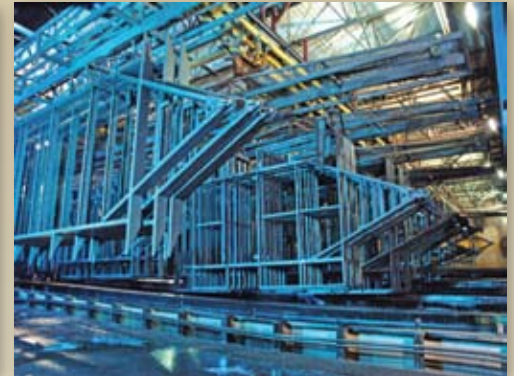
All Outback's are made with I-Beam chassis and full size outriggers. Pretreated in an 11 step process prior to painting ensures more rust resistance than our competitor's chassis.
