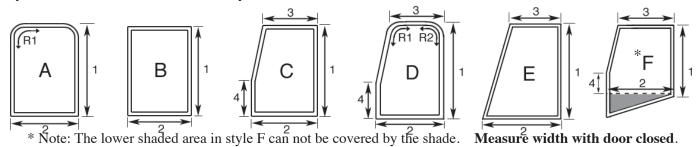
Measure the indicated areas of the screen door frame. Example: If your screen door frame shape is style A, you would write style "A" on the form below and then include measurements for 1 and 2 and radius 1 (R1) on the form. Measure the outside of the frame to the outside of the frame. For an example, see photo of Style A. For Styles A and D, use the radius template on this page to determine the curvature of the door frame.
