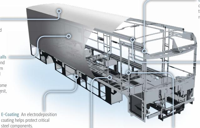
**Laser-Cut Tubing** Precision laser cutters create precise joints in structural steel that are stronger and require less welding.
