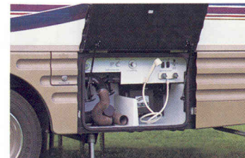
34Y This compartment is packed with convenience, including a wash station, swivel drain and sewer hose, city water hookup and TV cable as well as phone and cable TV input jacks.
