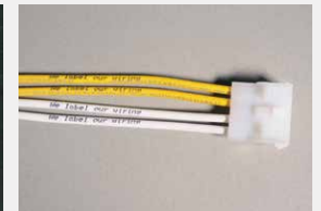
Wiring labeled and spliced to automotive standards
