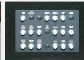
Resettable circuit breakers eliminate fuses
