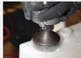
Holding tank fittings are spin-welded for water-tight connections
