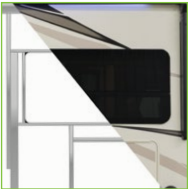
Aluminum Framing Around Windows in Sidewall
