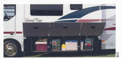
Thanks to Winnebago Industries' ingenious SIDR: MORE Hydraulic Slideout System, exterior storage space is plentiful. The unsurpassed, rugged design of the StoreMore system allows for full-length, full-height compartments which extend with the room — a feature most slideouts cannot offer.
