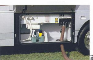
Separate water and electrical service centers neatly contain all controls and hook-ups in large compartments for increased work space. A second monitor panel, located in the water service center, allows quick and easy readings of tank levels.
