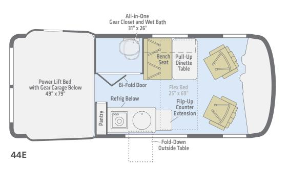
Storage and living space are maximized by the flared body and Power Lift Bed. Welded aluminum cabinet face frames, dual-pane windows with insulated shades, snap-in screens, and an available roof-mounted A/C system all contribute to the 44E's off-grid livability.
