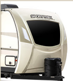
One-piece full fiberglass painted front cap includes integrated tinted high-end automotive glass front window, which provides privacy and panoramic views.
