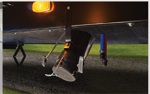
Termination Valve Service Light Standard on all models, this light allows adjustments to be made with two hands, no flashlight required.
