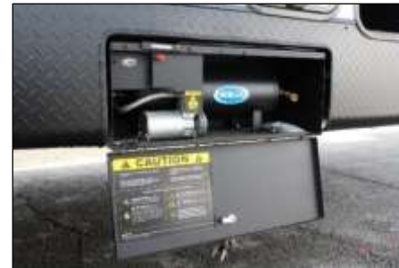
12-Volt On-Board Air Compressor
