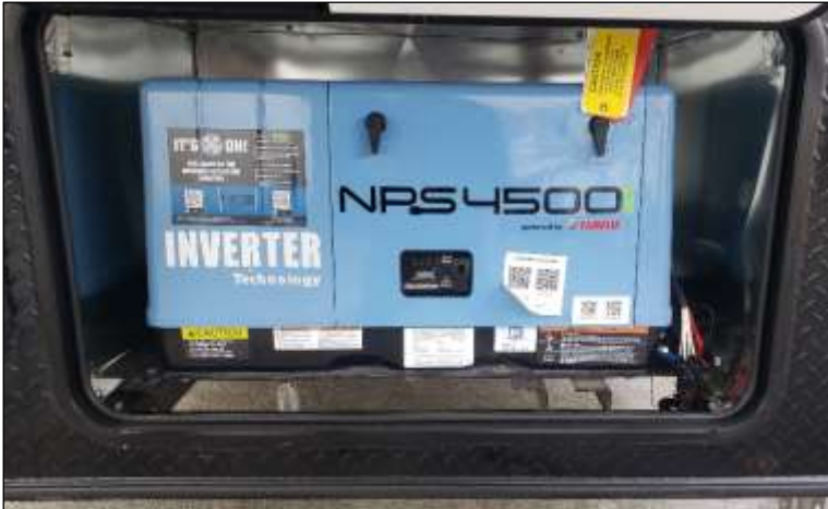
Yamaha 4.5KW Generator (Optional 6KW is similar)
