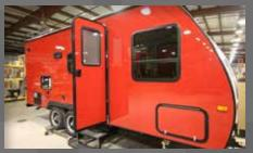
Our Noble Classic high gloss fiberglass sidewalls are manufactured with the supporting underlayment imbedded to the resin for a superior bond. This is the same process we use on our prestigious motor homes.
