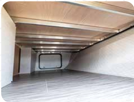
WELDED ALUMINUM BED FRAMING (16/19 SERIES ONLY)
