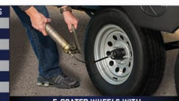
E-COATED WHEELS WITH E-Z LUBE AXLES
