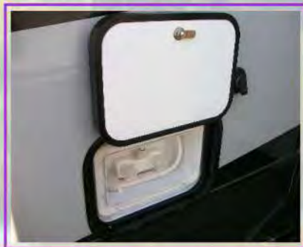
Exterior Shower Insulated by 1" Thick Thermal Insulated Luggage Door
