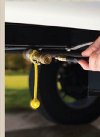
LP gas hook up
