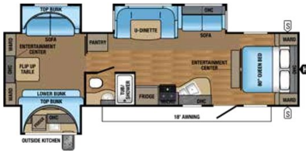
JAY FLIGHT | 32TSBH OPTION D Ext. Lgth: 36' 2" Ext. Ht: 134" Unloaded Wt (lbs.): 8,240 Sleeps: 9-11
