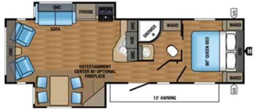
JAY FLIGHT | 29RLDS OPTIONS: D, E Ext. Lgth: 33' 2" Ext. Ht: 136" Unloaded Wt (lbs.): 6,735 Sleeps: 2-4
