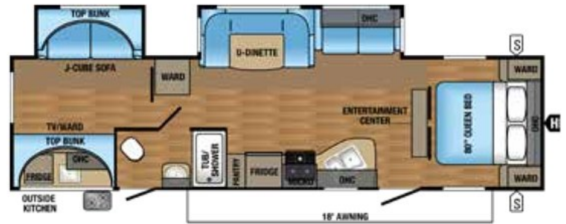
JAY FLIGHT | 32BHDS OPTION D Ext. Lgth: 36' 2" Ext. Ht: 135" Unloaded Wt (lbs.): 7,595 Sleeps: 8-10
