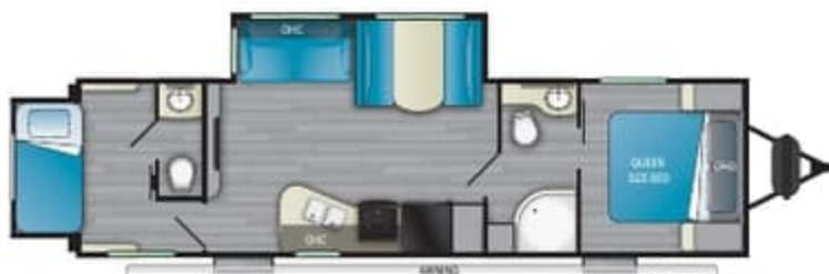
SD 283RB Length - 34' 9" Dry - 6,920 lbs. Hitch - 820 lbs. Height - 11' 2" GVWR 9,620 lbs.
