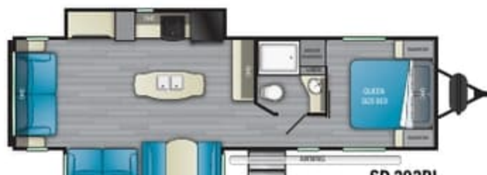
SD 293RL Length - 34' 2" Dry - 7,069 lbs. Hitch - 954 lbs. Height - 11' 2" GVWR 9,754 lbs.
