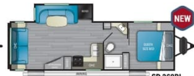
SD 268RL Length - 30' 11" Dry - 5,800 lbs. Hitch - 800 lbs. Height - 10' 11" GVWR 7,800 lbs.
