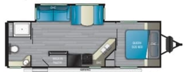
SD 262RB Length - 30' 10" Dry - 5,920 lbs. Hitch - 780 lbs. Height - 10' 11" GVWR 7,780 lbs.
