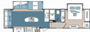
DENALI FIFTH WHEEL | 335RLK Ext. Length: 37' 6" Ext. Height: 13' Average Shipping Weight: 9,929 Sleeps: 8
