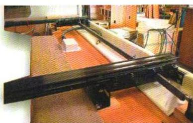
Dual Ram Gear Driven Slide Assembly in All Slide Outs
