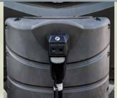
The power tongue jacks allow you to adjust your trailers hitch height with the push of a button.
