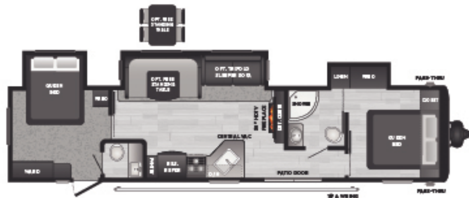
38FQTS | Three slides, double queen bedroom, 1½ baths, patio door Weight: 9230 lb | Length: 39' 11"
