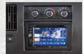
Dash stereo with touch screen control and integrated back-up monitor. (Lead Dog Package)
