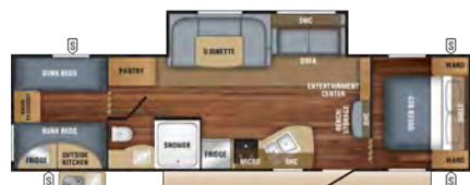
JAY FLIGHT SLX | 294QBS OPTION A Ext. Lgth: 35' 5" Ext. Ht: 133" Unloaded Wt. (lbs): 6,480 Sleeps: 8-10
