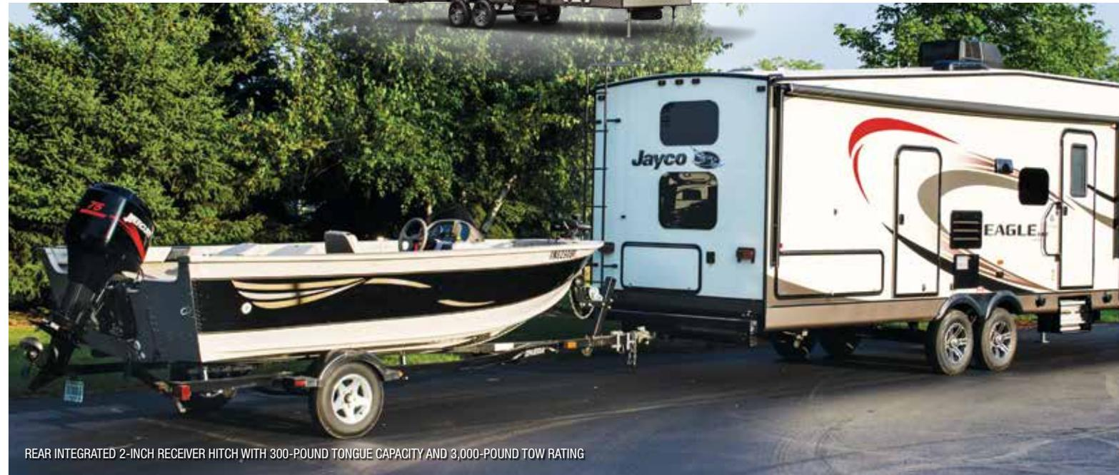
REAR INTEGRATED 2-INCH RECEIVER HITCH WITH 300-POUND TONGUE CAPACITY AND 3,000-POUND TOW RATING
