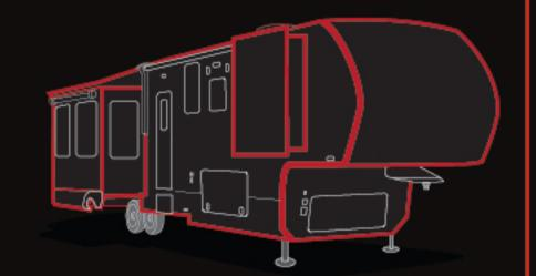
Utilizing Mylar Tape and Die-Cut Seals at ALL critical seams (roof to sidewall, floor to sidewall and backwall to sidewall).
