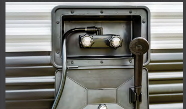
Outside Shower with Hot and Cold Water
